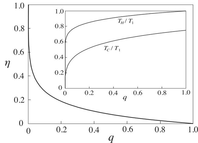
Fig. 2. Efficiency  $\eta$  as a function of the hot area fraction  $q$  for optimized power, according to Eq. (9). Inset: temperatures of the hot and cold surfaces as functions of  $q$ .
